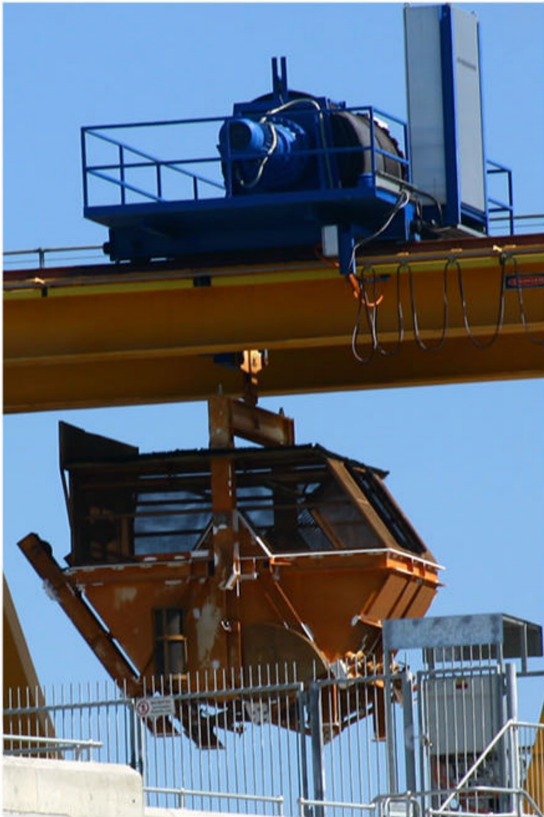
Image 9: Close-up of fishlift not in operation on top of Paradise Dam wall. Taken by Arkin Mackay, August 2006.
